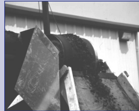
Asphalt shingles processed into 1/2" minus particles, ready for transport to asphalt plant.
