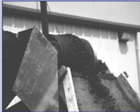
Asphalt shingles processed into 1/2" minus particles, ready for transport to asphalt plant.
